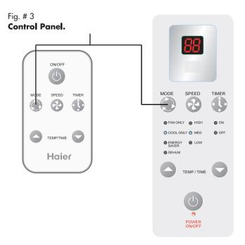
Once the mode function is established, you will have to set the fan speed. (See fig. #4) Every time you press the SPEED button, fan speed will change between LOW, MED, and HIGH.
